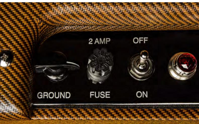
Located next to the Fuse Holder is the VAC control (GROUND). This is a built in attenuator. Its purpose is to allow the Volume controls to be turned up to achieve the desired sound, but then reduce the overall volume level with the VAC, retaining the turned up sound.
